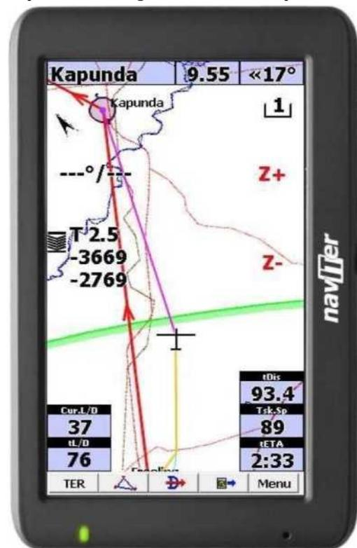
Figure 2 - Oudie flight computer with simple uncluttered display
