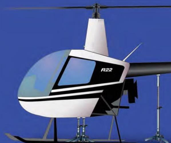
$$\begin{aligned} \text{CG inches from datum} &= \text{LEMAC} + \frac{\text{MAC} \times \text{CG \% MAC}}{100} \\ &= 144 + \frac{62 \times 27.4}{100} \\ &= 160.9 \end{aligned}$$
