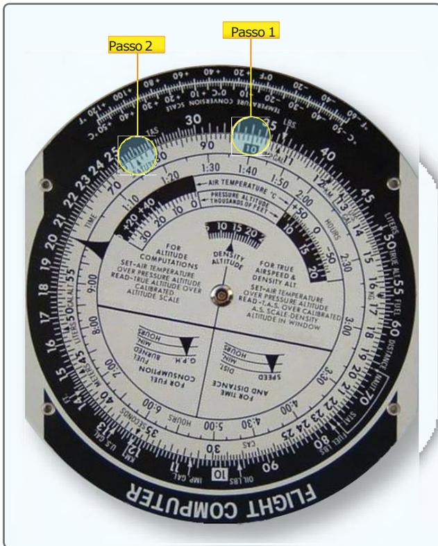
Figure 10-3. E6-B computer set up to multiply 340 by 78.
